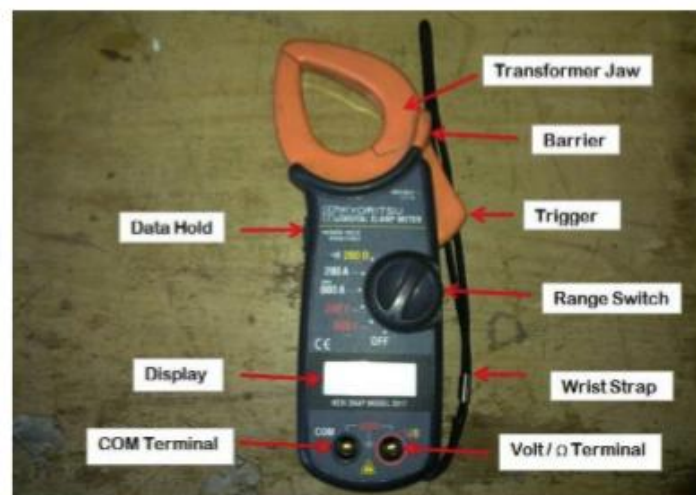
Gambar 4 . Bagian-bagian Tang Ampere
