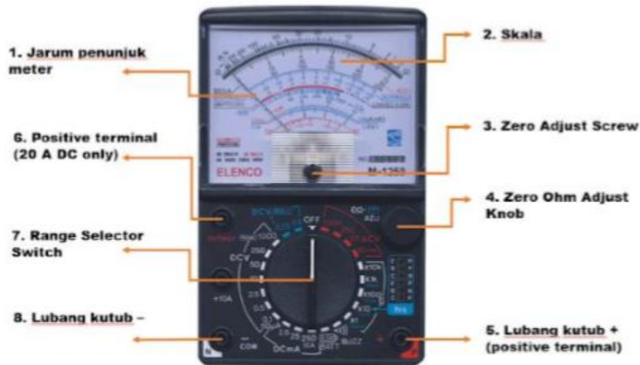
Gambar 2 . Bagian-bagian Multimeter Analog
